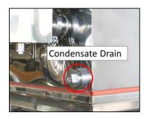
19. Using  $1 - \frac{1}{2}$ " fittings (not supplied), connect to the condensate drain. It is best to use stainless steel or copper plumbing and fittings. The condensate can either be sent to drain or collected for use in the sugar house. The drain end must be open at all times. Do NOT submerse the end of the drain or allow the drain pipe to sag and fill with condensate.
