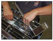
b. Begin inserting the float into the float box while holding up the regulator arm. The float should be angled slightly toward the outside of the float box (away from the flue pan) and lengthwise on end to be able to slide under the regulator arm. The regulator arm will be on the flue pan side of the float stem.
