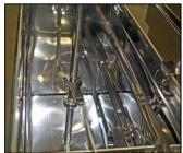
d. Rotate the float toward the rear of the float box until the regulator fork will slide around the float stem over the adjustment ring. Lower the float back to the bottom of the float box.
