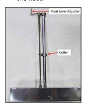
a. Turn the float level adjuster until the collar is about halfway on the rod.
