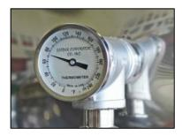
21. If not included in the evaporator package the temperature of the sap exiting the Steam-Away can be monitored with a thermometer. To install the thermometer, remove the ¼" stainless steel plug from the stainless steel tee connected to the Steam-Away. Wrap the threads, with Teflon tape, of a thermometer (Leader Order #: 61019) and thread and tighten into the tee.
