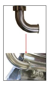
16. Using the 4" clamp and 4" TEFLON gasket, install the air injector adapter onto the Steam Away. It can be installed on either side depending on which side is best suited for connection to the blower. NOTE – install the 4" cap on the side opposite the side the adapter installed.
