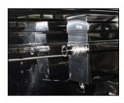
7. Install the flue pan Sap Regulator Float Box adapter into the side of the flue pan regulator box. Tape the threads and securely tighten into the threads in the side of the regulator box.
