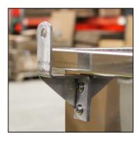
b. Use two ¼" X ¾" stove bolts and ¼" hex nuts for each hanger, attach to the Steam-Away. The bracket should point up vertically. Tighten securely.
