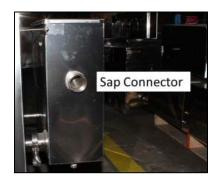
20. Connect the sap source to the sap regulator float box. Ensure you have a shut off valve between the sap source and the float box. The following is a recommended method of attaching the sap source to the regulator box. The items for this connection as shown are not included with the evaporator.
