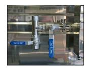
8. Install the flue pan regulator box assembly to the flue pan regulator box. The assembly is clamped to the float box adapter installed in the previous step. The assembly should be positioned vertically with the drain oriented down.
