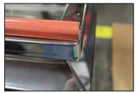
5. Remove the top backer of the adhesive seal and press the rubber gasket into place on the adhesive.
