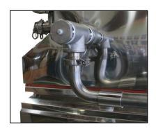
13. Connect the flanged end of the connection pipe to the flange of the outgoing tee assembly using a clamp and Teflon gasket.
