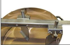
4. Position the paddles about ½" from the bottom of the paddle bar then tighten the thumbscrew to hold the paddles. Place the paddle bar on the base pins. Lock the paddle bar in place using the snap locks inserted into the outer holes on the top of the paddle bar.
