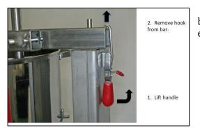
1. Remove the assembled paddle bar and paddles from the base by lifting up on the fasteners to unhook them from the bar ends. Lift the paddle bar assembly straight up off the pins.
