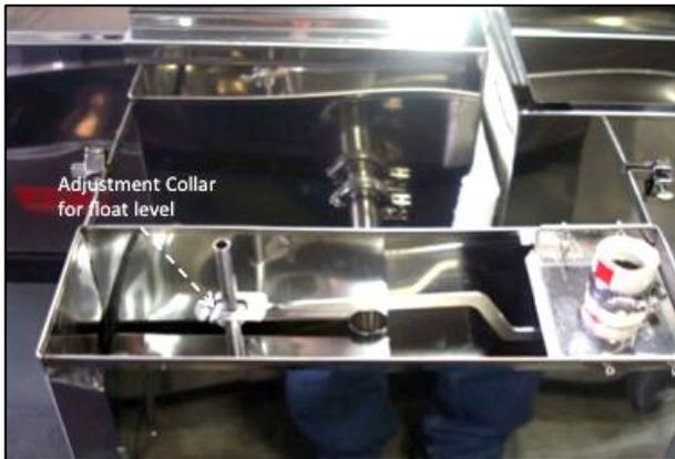
1. Set the float so the level of sap over the flues is 1" in depth. To set the depth using the float, loosen the thumbscrew on the side of the float shaft collar. Raise the collar to lower the level of the sap. Lower the collar to raise the level of the sap. Tighten the thumbscrew when the proper level is set.
