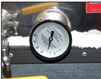
18. It is recommended a thermometer be installed. The thermometer is used to aid in determining when the boiling sap has reached the conditions for draw off. To install the thermometer, remove the 1/4" plug in the coupler on the draw off side of the syrup pan. Teflon tape the threads of the thermometer then thread the thermometer into the 1/4" coupler. Tighten the thermometer so the "7" on the thermometer is on the bottom.
