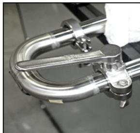
NOTE: LEADER EVAPORATOR offers an upgrade to the WSE (LEADER EVAPORATOR part number 390002). The kit replaces the u-tube with a connector including a butterfly valve. The valve can be closed and the flue pan does not need to be drained when doing reversals or work on the syrup pan. This lessens the effects on the gradient in the evaporator.
