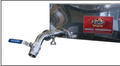
13. Install the draw off valve assembly. The draw off assembly should be as vertical as possible with the open end pointed down.
