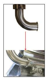
14. Using the 4" clamp and 4" TEFLON gasket, install the air injector adapter onto the Steam Away. It can be installed on either side depending on which side is best suited for connection to the blower. NOTE – install the 4" cap on the side opposite the side the adapter installed.
