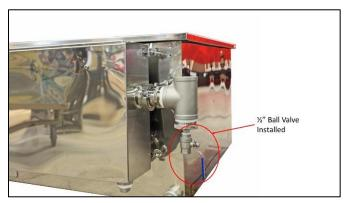
22. Thread the ½" stainless steel ball valve and nipple assembly into the adapter in the bottom of the tee and tighten all parts into the tee (adapter, nipple, and ball valve). . Make sure the handle of the ball valve can operate without interference.
