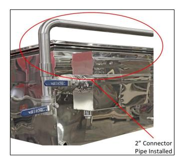
Install the connection pipe to the flue pan regulator box assembly by clamping onto to hot sap feed assembly.
