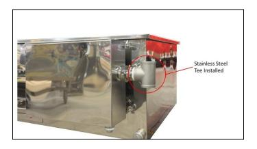
20. Thread the 2" stainless steel "tee" onto the threaded end of the adapter and tighten until the open ends are straight up and down.
