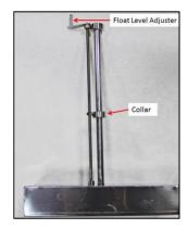
a. Turn the float level adjuster until the collar is about halfway on the rod.
