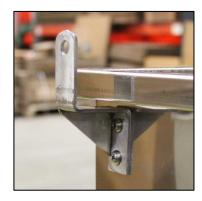
b. Use two ¼" X ¾" stove bolts and ¼" hex nuts for each hanger, attach to the Steam-Away. The bracket should point up vertically. Tighten securely.
