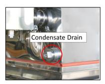
b. Ensure the condensate drain is flowing. Note installation of a  $1 - \frac{1}{2}$ " nipple and ball valve prior to use will aid in draining the condensate.
