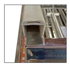
3. Install the gasket by slipping the U over the top lip of the flue pan.
