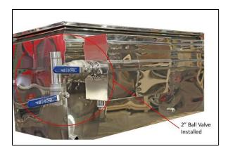
7. Install the flue pan regulator box assembly to the flue pan regulator box. The assembly is clamped to the clampable fitting on the side of the flue pan regulator box. The assembly should be positioned vertically with the drain oriented down.
