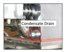
17. Using  $1 - \frac{1}{2}$ " fittings (not supplied), connect to the condensate drain. It is best to use stainless steel or copper plumbing and fittings. The condensate can either be sent to drain or collected for use in the sugar house. The drain end must be open at all times. Do NOT submerse the end of the drain or allow the drain pipe to sag and fill with condensate.
