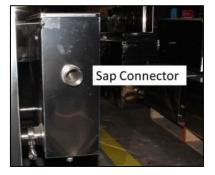
18. Connect the sap source to the sap regulator float box of the steam away. Ensure you have a shut off valve between the sap source and the float box. The following is a recommended method of attaching the sap source to the regulator box. The items for this connection as shown are not included with the evaporator.
