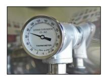
19. If not included in the evaporator package the temperature of the sap exiting the Steam-Away can be monitored with a thermometer. To install the thermometer, remove the ¼" stainless steel plug from the stainless steel tee connected to the Steam-Away. Wrap the threads, with Teflon tape, of a thermometer (Leader Order #: 61019) and thread and tighten into the tee.
