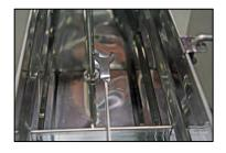
c. Continue to rotate the float downward and under the regulator arm until the float is resting on the bottom of the float box. The regulator arm will be on the side of the float stem.
