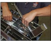
b. Begin inserting the float into the float box while holding up the regulator arm. The float should be angled slightly toward the outside of the float box (away from the flue pan) and lengthwise on end to be able to slide under the regulator arm. The regulator arm will be on the flue pan side of the float stem.
