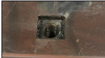
1. Insert a thumbscrew assembly into each of the locations provided on the arch. They are located on the front top of the arch above the control panel.
