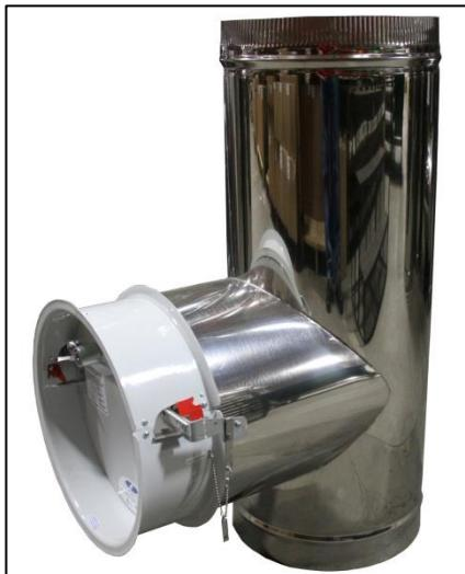
1. The first stack section is the section having the barometric damper installed. Place it on the collar of the arch. NOTE: If the pans have not been installed ensure the barometric damper is positioned so it will not hit the flue pan.
