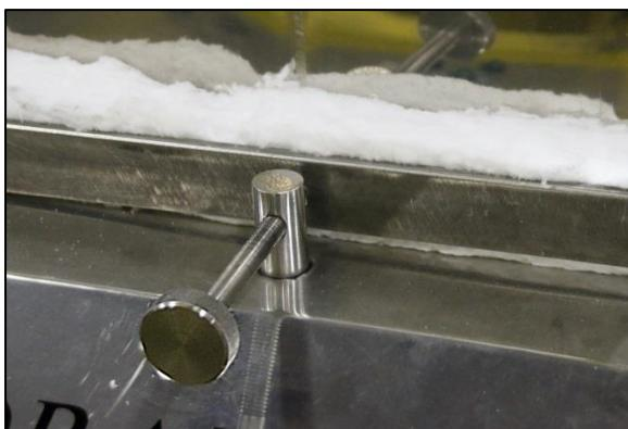
4. Tighten the thumbscrews to secure the rail gaskets of the pan sets.
