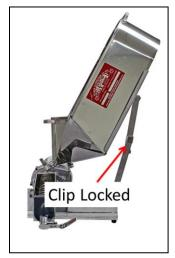
7. Support the "pig" platform and slide the locking clip on the "pig" holder hinge up.
