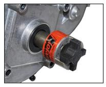
3. Insert the 4-way coupling spider into the coupling on the motor shaft. The fingers of the spider go around the projections of the coupler
