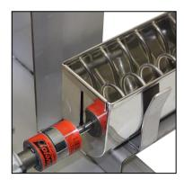
6. Put the slide gate inside the end of the trough where the worm shaft is cut. Slide the gate down until it is seated on the edge of the trough.
