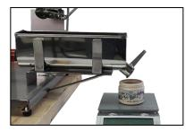
11. To draw off the cream slowly open the spigot end of the trough. As you do so, slightly open the valve in the end of the pig to slowly replace the volume of cream being drawn.
