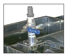
9. Teflon tape the threaded end of a 1" PVC adapter (not included) and thread it into the open end of the ball valve. Tighten.
