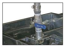
10. Obtain a length of 1" braided hose (not included) of sufficient length to reach from the sap source and onto the 1" PVC adapter. Secure the hose on the PVC adapter with a 1" stainless steel band clamp (not included). Connect the other end of the hose to the sap source.
