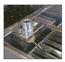
5. The L shaped part of the bolt on assembly should be placed on the outside of the pan. The top of the L shape has cutouts for the incoming sap connection and the screws. These cutouts should be aligned with the section of the bolt on regulator and the screws. The screws should be partially threaded in place.
