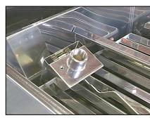
4. Position the section with the float arm into the pan compartment as shown in the location drawing. It should be parallel to the side of the pan and approximately in the center of the compartment.
