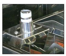
7. Telon tape the threads on both sides of a 1" stainless steel close nipple (not included). Thread the nipple into the top of the bolt on regulator assembly.
