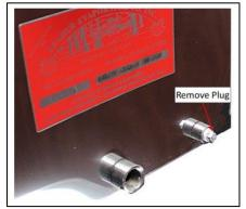
Remove the stainless steel plug from the ¼" threaded coupler.
