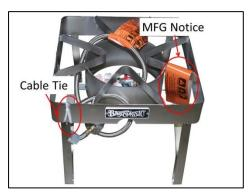
3. Turn the burner so the end is outside of the frame of the arch and are approximately 90 degrees to the frame. Tighten the 10MM fastener bolt located under the burner to secure the burner in place. Failure to remove the cable tie and properly position the burner will result in damage to the unit.
